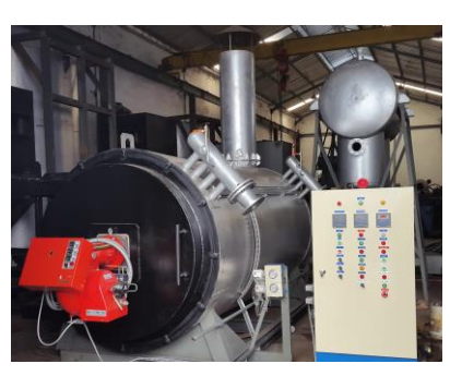
Boiler for Tanker Ship
